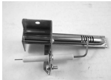
Figure (25) Spark Probe Adjustment
